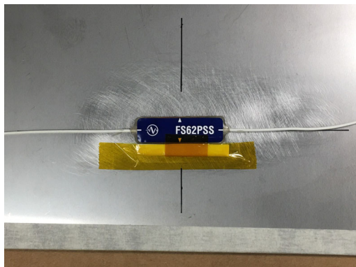
Fig. 2.9 Aligning and placing the FS62PSS
