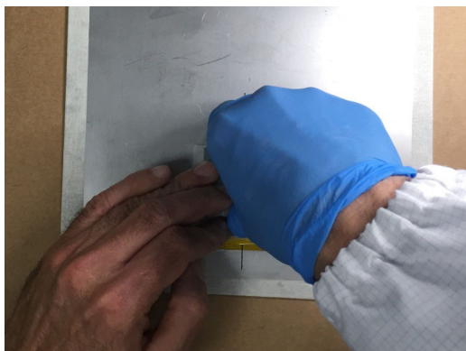
Fig. 2.22 Pressing on the rosette for 1 minute
