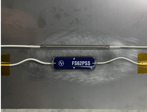
Fig. 2.25 Positioning the temperature sensor
