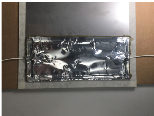
Fig. 2.35 Completely covered measuring point
