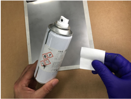
Fig. 2.4 Using RMS1 cleaner and nonwoven tissues
