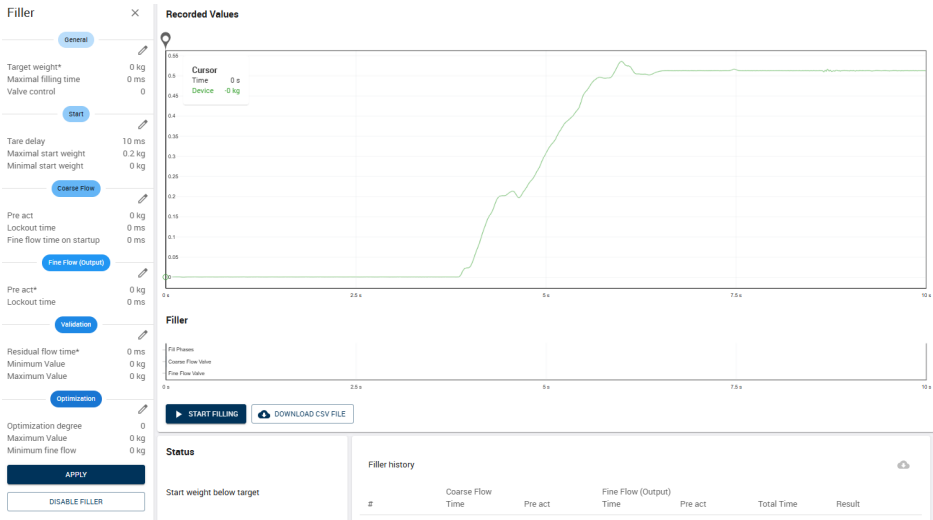
Fig. 7.30 Sequence of a filling process (example)
