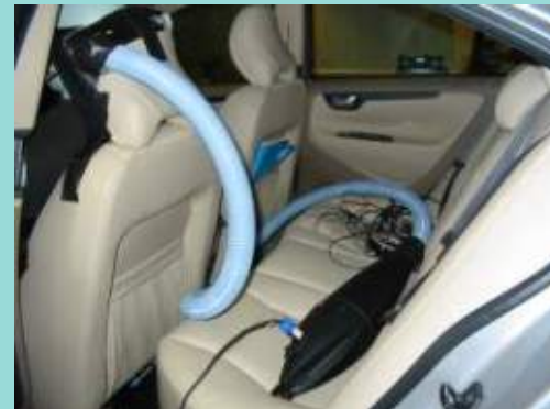
Reciprocal method using volume velocity source
