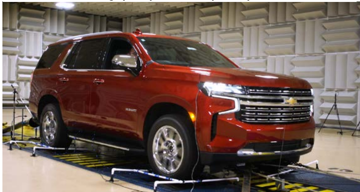
Indoor Pass-by propulsion (PTN) noise
