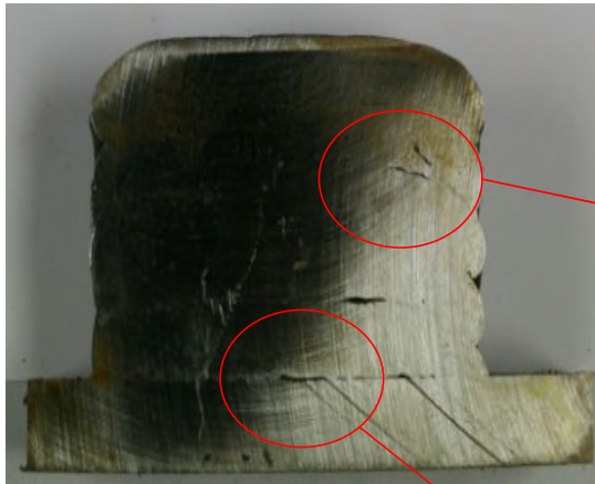
Lack of fusion
