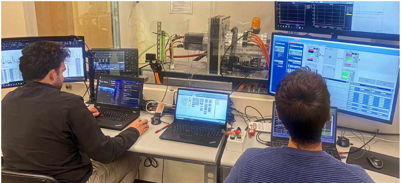
H3X engineers performing dynamometer testing and characterization with the HBK eDrive system and Perception software.
