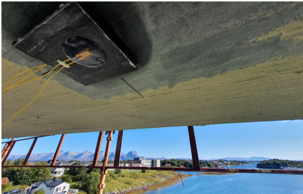
Strain gauge with temperature compensation (the Seven Sisters mountain range can be seen in the background)
