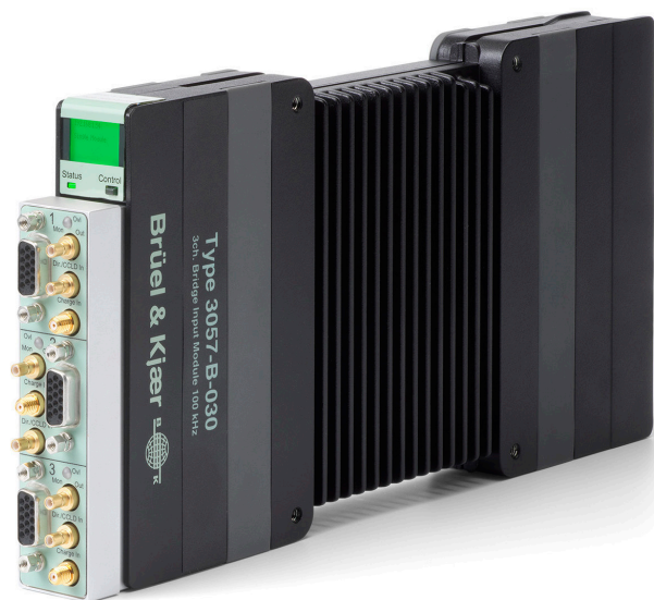
Figure 1. LAN-XI Bridge Input Module with three channels, 0 – 100 kHz measurement bandwidth.
