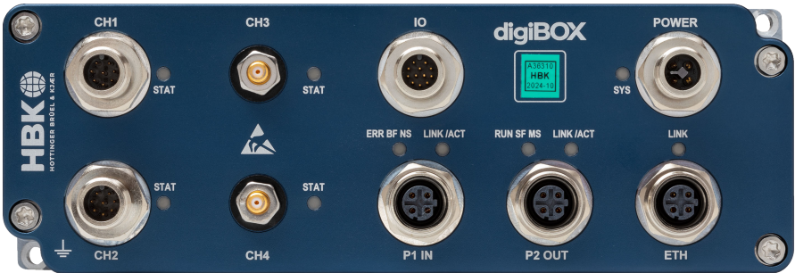
Fig. 3.2 Overview of digiBOX Industrial connections (configuration shown: K-DBX-4M-AD-IE-I-ILT)
