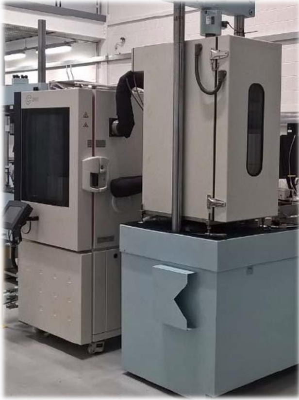
Environmental conditioning chamber with satellite test chamber: -40C to 150C dry, RT to 80C up to 85%rH
