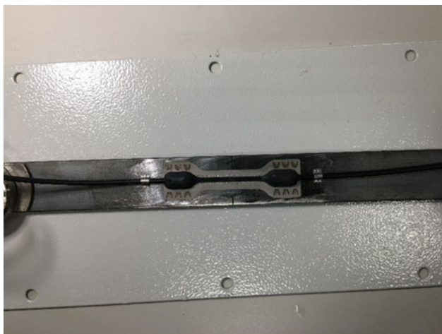
Fig. 2.21 Welded sensor with steel clips
