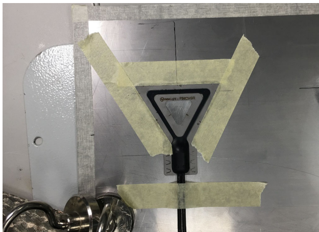
Fig. 2.25 Aligned and tape secured FS62WSR
