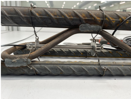
Fig. 2.4 Sensor in place between the bars
