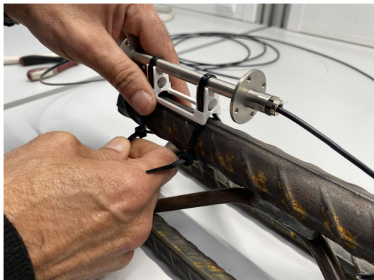
Fig. 2.7 Securing the sensor to the bar
