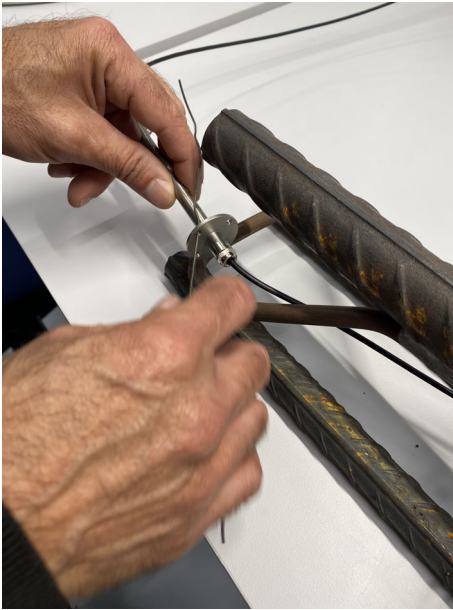
Fig. 2.3 Threading the securing wire
