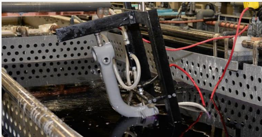
Landing Gear Component Set Up for Zinc-Nickel Plating 1
