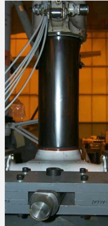
Application of HVOF Coating to Landing Gear Component (Left); After grinding/finishing (Right) 1
