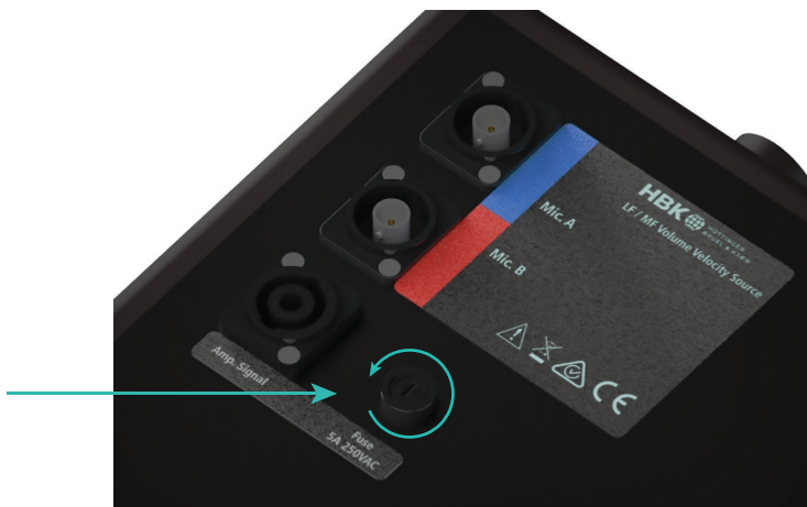
Fig. 5.1 Location of the fuse holder. Turn anti-clockwise to open
