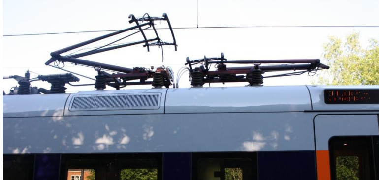
Fig. 5. Picture of pantograph on Oresund train. The train is driving to the right, and the front pantograph is folded
