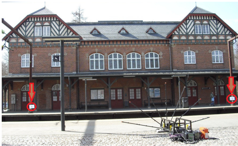
Fig. 2. Half-wheel microphone array (with 42 channels) on the platform at Skodsborg Station, Denmark. Two photo-cells were used for position calculation (indicated with red arrows).
