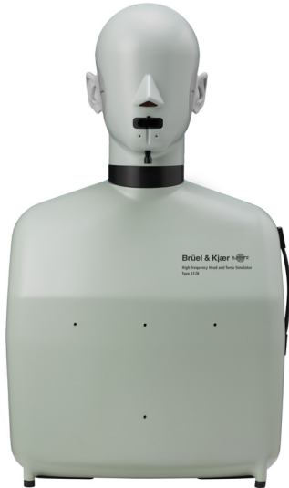
HBK High-frequency HATS Type 5128 enables binaural recordings that accurately capture how electrified aircraft are perceived by listeners.
