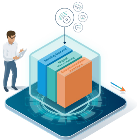
Modern setup: In-line integrated amplifier – the complete measurement chain reduced to one single unit
