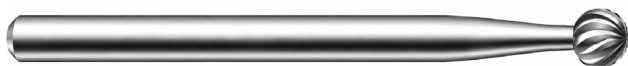
Fig. 3.41: Carbide dental burr (roundhead milling cutter) for cutting PCB board conductors. The head should have a diameter of approx. 0.8 mm (shown enlarged)
