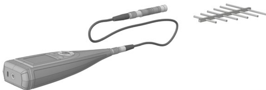
Fig. 3.2 Reference orientation of the sound level meter relative to the RF-emitter/receiver
